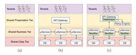
**Fig. 1.** Overview of application-level multi-tenancy (a) for both microservice applications (b) and applications with ThunQ (c). ThunQ's components are shown in green.
